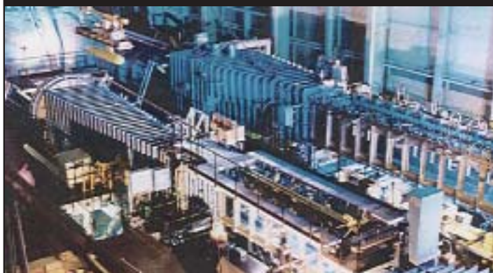
DCN cavitation tunnel in Val de Reuil used for testing our propellers
